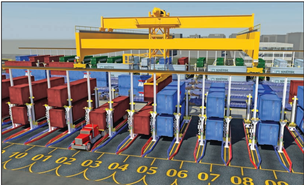
Figure 1: A 2-High ATMS Positioned Perpendicular to the Tracks, with WSG Crane and Loading Tracks in the Background
